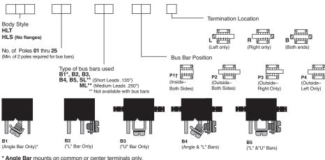
Angle Bar mounts on common or center terminals only. †Min
